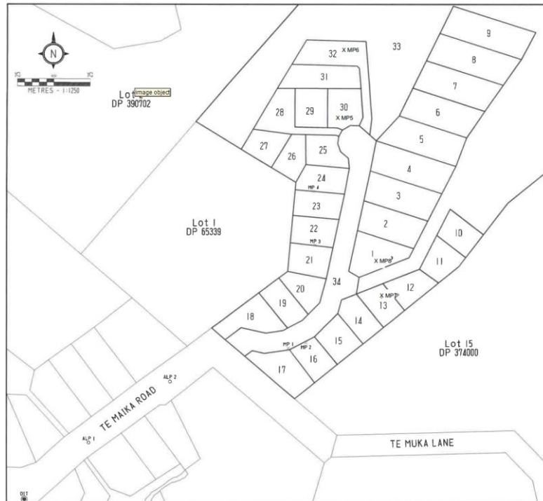
Figure 2 - View of subdivision showing location of settlement pads (Source R&B Ltd)
